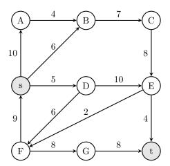
Question 3.1 (7%) Give a maximum flow from s to t in the network N (write the flow for each edge along the edges on the graph below), give the value of the maximum flow, and give a minimum s-t cut (give the partition of the vertices).
