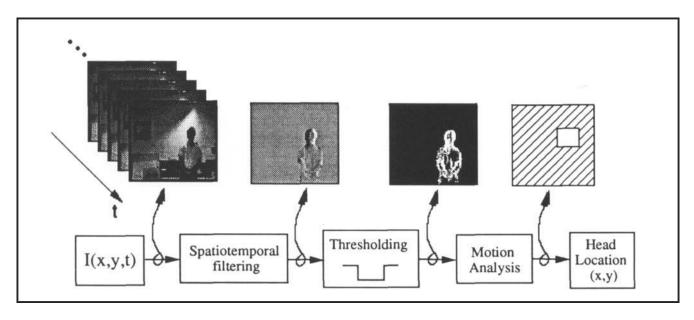
Figure 5. The head tracking and locating system.
