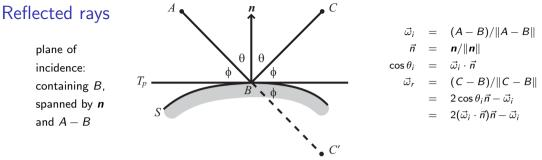
Light path from A to C by reflection off a mirror surface S.
