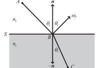
$$\begin{aligned} \cos \theta_i &= \vec{\omega}_i \cdot \vec{n} \\ \sin^2 \theta_i &= 1 - (\vec{\omega}_i \cdot \vec{n})^2 \\ \sin \theta_t &= \frac{n_i}{n_t} \sin \theta_i \\ \cos^2 \theta_t &= 1 - \left(\frac{n_i}{n_t}\right)^2 (1 - (\vec{\omega}_i \cdot \vec{n})^2) \\ \vec{t} &= \frac{\cos \theta_i \vec{n} - \vec{\omega}_i}{\sin \theta_i} \\ \vec{t} \sin \theta_t &= \frac{n_i}{n_t} ((\vec{\omega}_i \cdot \vec{n}) \vec{n} - \vec{\omega}_i) \end{aligned}$$
