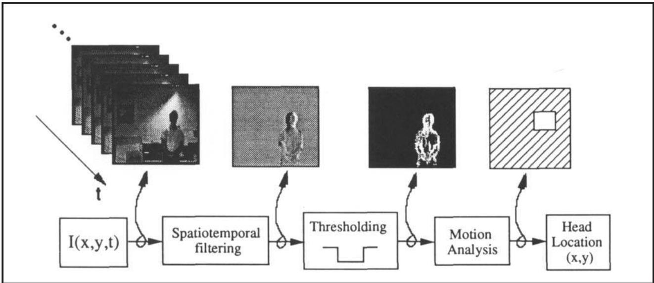
Figure 5. The head tracking and locating system.
