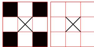
Figure 3: Left: SE1, Right: SE2. White pixels are foreground (1) and black pixels are background (0). The center is marked with a cross.
